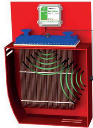
Above - Typical box cooler setup
